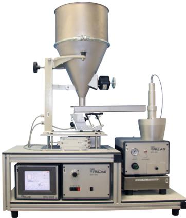
The refilling system, with a dosing unit and large storage container (see illustration), ensures continuous dispersion without interruption over several days.
