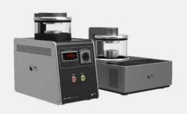
The Ion Sputter Coater allows for imaging of nonconductive samples in high vacuum mode for the highest resolution imaging. Sputter coaters increase conductivity by coating the test specimen with a few nanometer thick metal film of Au or Pt. The higher conductivity increases the amount of secondary electron generation and creates higher resolution images.
