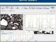
The line scan mode provides comparative elemental analysis along a user defined line with element profiles graphically representesd. Great for cross section thickness and elemental transition mizing studies.
