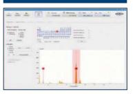
Acquire fast and accurate qualitative or quantitative analysis results with automatic peak deconvolution providing higher accuracy and reliable results for the defined area or point of interest.
