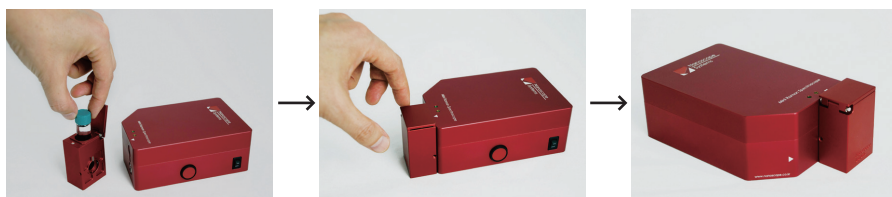
Quick and convenient measurement with vial holder
