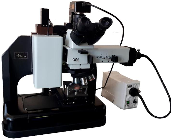
NIOS Micro is a new device in the NIOS product line that is designed to perform Vickers micro-indentation in the scale range from HV 0.01 to HV 50. It is certified as a measuring instrument and can be used in scientific and industrial laboratories.
