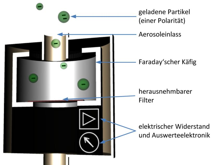
Fig. 1: Principle of operation of the Charmé<sup>®</sup> aerosol electrometer
